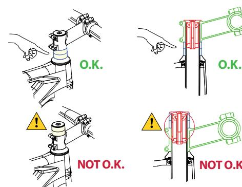
**⚠** Never install headset spacers above the stem. Placing spacers above the stem, especially on forks with a carbon steerer tube, can cause the expander inside the fork tube to be positioned above the lower limit of the steerer tube, which can stress the materials beyond the use for which they were designed, possibly causing accidents and serious injuries.
