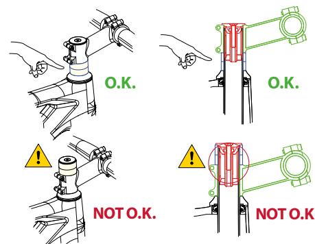
**⚠** Never install head tube spacers above the stem. Placing spacers above the stem, especially on forks with a carbon head tube, can cause the head tube expander inside the fork tube to be positioned above the lower limit of the head tube, which can stress the materials beyond the use for which they were designed, possibly causing accidents and serious injuries.
