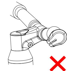
3. Once the fixing bolt is torqued to 0.5 N.m, it is normal that the plugs can be turned on the handlebar if sufficient force is applied. This is a safety feature to avoid damage to the components in case of a crash or a fall.
