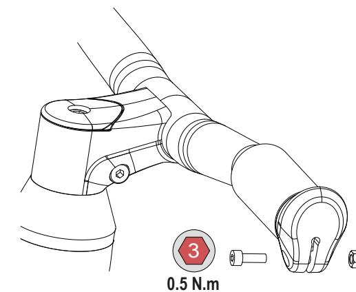
2. The plugs must be positioned on the handlebar so the slit is oriented downwards.
