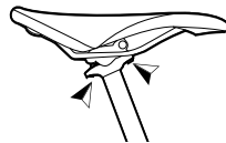
Figure 7. Saddle with two fitting blocks
